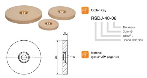
The drylin® slide disks from stock (RSD = Round Slide Disk) made of high performance material iglidur® J have many different applications. Without additional lubricant, heavy loads can be moved over a variety of surfaces (steel, aluminum, stainless steel, etc.) with very low friction. The plates are fixed securely with a screw through the reinforced hole in the centre.
