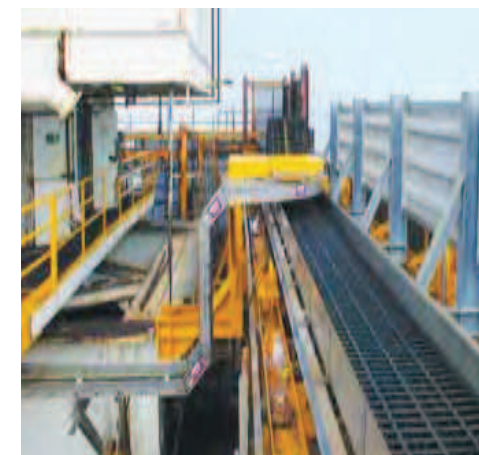
Rig skidding application on the Claymore, North Sea
