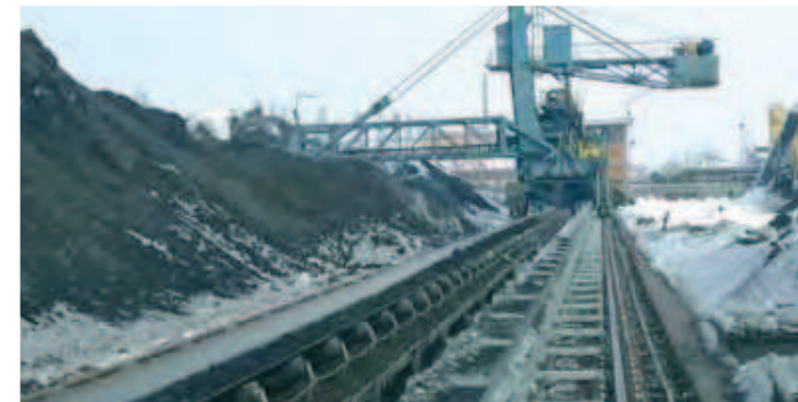
180 m travel, 30 kg/m fill weight. Two igus® E4 rol e-chains®
