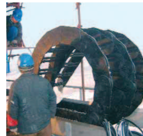
Assembling of an E4 e-chain® Series 800 in an igus® steel guide trough
