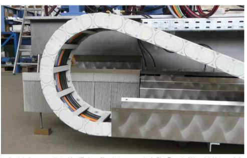
igus® e-chains® can even withstand the difficult conditions in stone processing facilities. The task of this e-chain® is to supply the tool carriage with energy (up to 100 A), signals, compressed air and water. It can travel up to 12m and achieves speeds of up to 32m/min.
