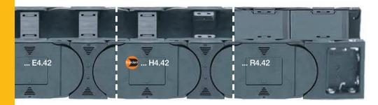
e-chains® | Series E4.42 | Crossbars every link (crossbars removable along the inner and outer radius) e-chains<sup>®</sup> Series H4.42 Crossbars every 2<sup>nd</sup> link (crossbars removable along the inner and outer radius) e-tubes | Series R4.42 | Fully enclosed (lids openable along the outer radius, from one side)
